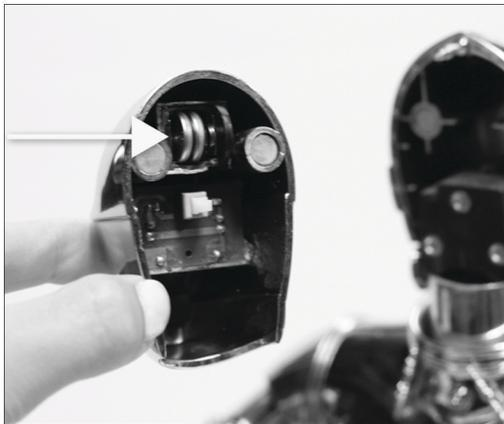
LED light up components: Remove C-3PO's face mask and suspend springs back to insert the two included CR1130 Lithium Coin Cell Batteries.
