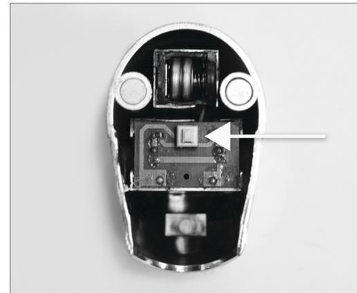
LED light up components: To turn on the light up feature, push the white power button under the battery area.
