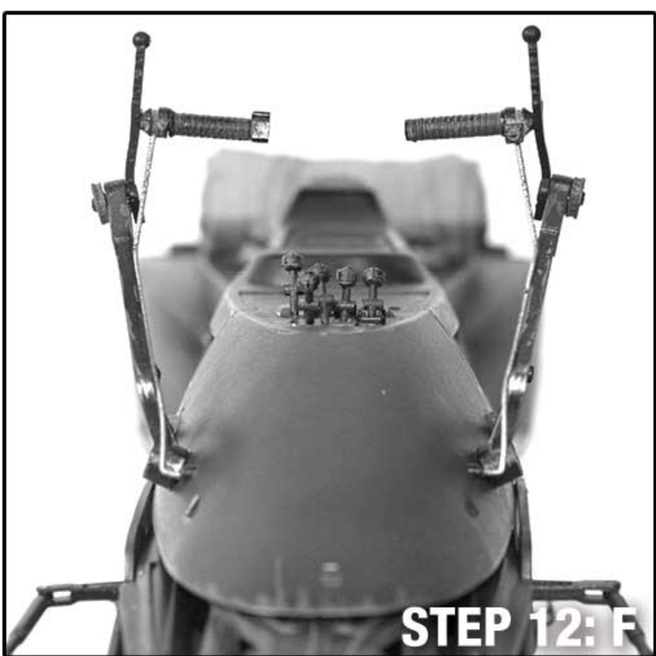
STEP 12: Install both left and right steering levers by plugging in the larger square key first. Due to a friction fit, slightly wiggle the larger square key into place. After the larger square key has been securely placed, slide the two softer cables into their designated slots. The softer cables are not a friction fit and will be loose fitting.
