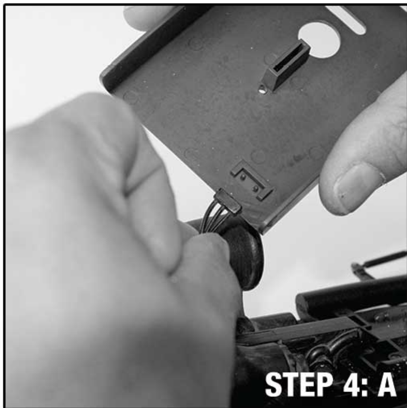
STEP 4: Plug the rectangular cap attached to the power cell recharging lines into the double prong slot located along the inside of the bottom protective armor. Key bottom protective armor into the matching rectangular key plug on the outrigger assembly.
