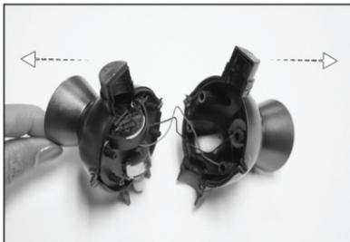
Gently pull apart Power Battery to reveal the CR2032 battery (do not pull too far to snap wires).
