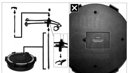
Assemble the figure stand in the steps as indicated. The clip is not recommended to remove as the battery holder can be separated as shown.
