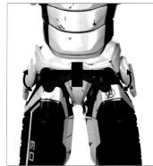
The flaps will push up automatically when moving the legs. It is suggested to extend the legs by pulling them down slightly for easier positioning.
