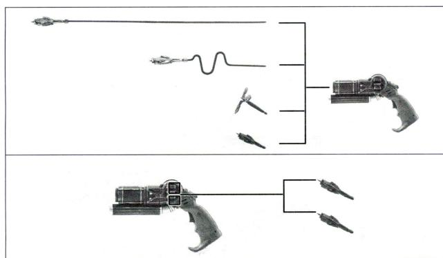
Four styles of grappling hooks can be interchanged and attached onto the grappling gun as shown. Two styles of grappling hooks in closed mode can be interchanged and attached onto the grappling gun as shown.
