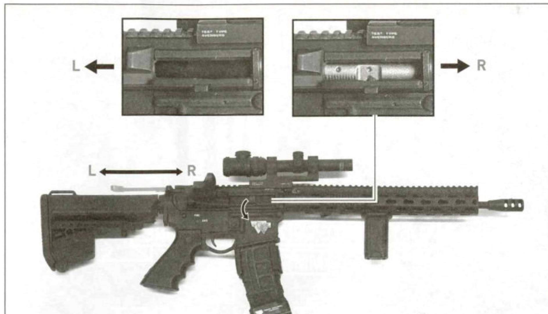
Hold the indicated part downwards to shift left or right as shown.
