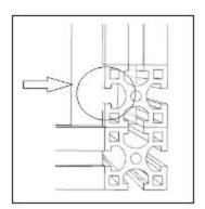
Insert rubber strip into slot
