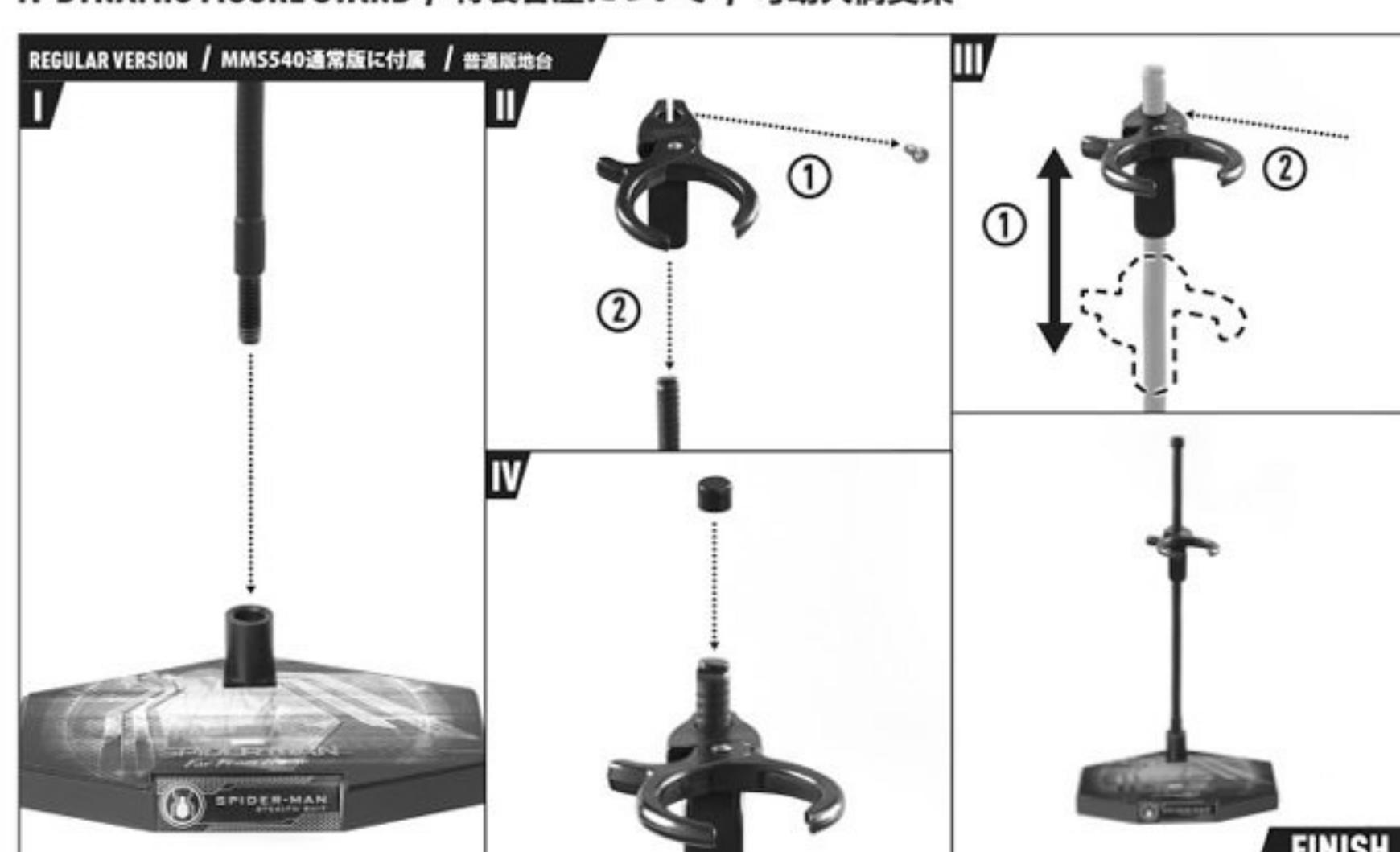
Follow the steps and attach the flexible poles and the figure holding clip to the base. Adjust the clip position before tightening the screw as indicated. Complete as shown.
