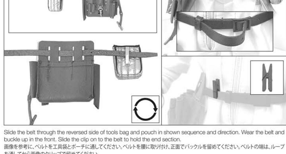
Slide the belt through the reversed side of tools bag and pouch in shown sequence and direction. Wear the belt and buckle up in the front. Slide the clip on to the belt to hold the end section.
