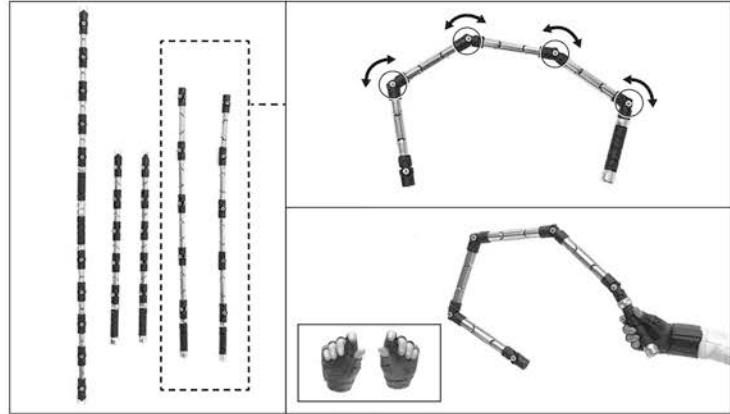
Three styles of baton. Indicated batons are equipped with articulated function. Use the indicated hands to hold the batons.
